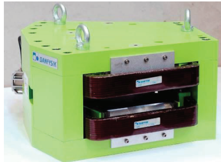
Figure 2: Photo showing our first AMS magnet based on Green Magnet technology.
